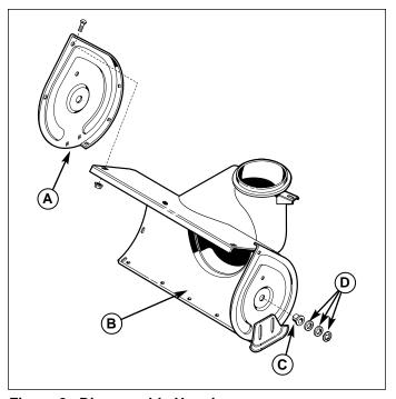
Figure 2. Disassemble Housing
